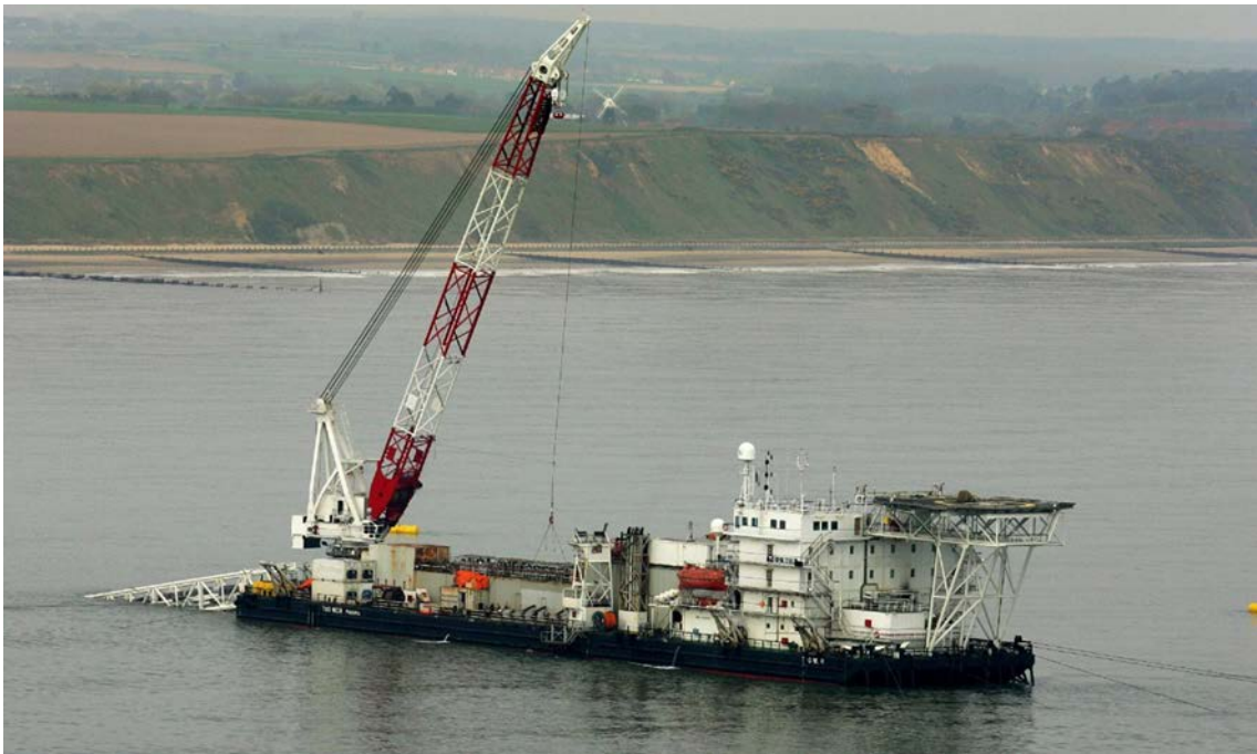
Figure 4.10: Typical S-Lay Vessel
