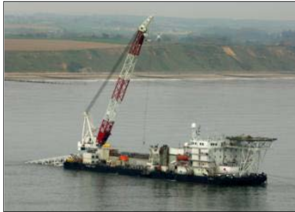
Figure 4: Example of Pipelaying Vessel
