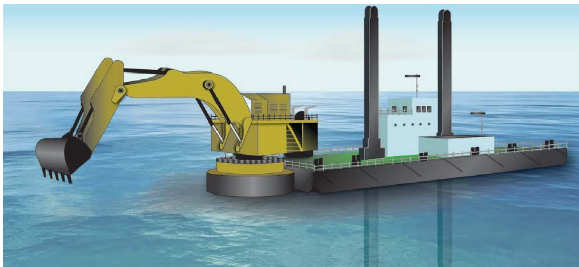
Figure 4.8: Schematic of Backhoe Dredger
