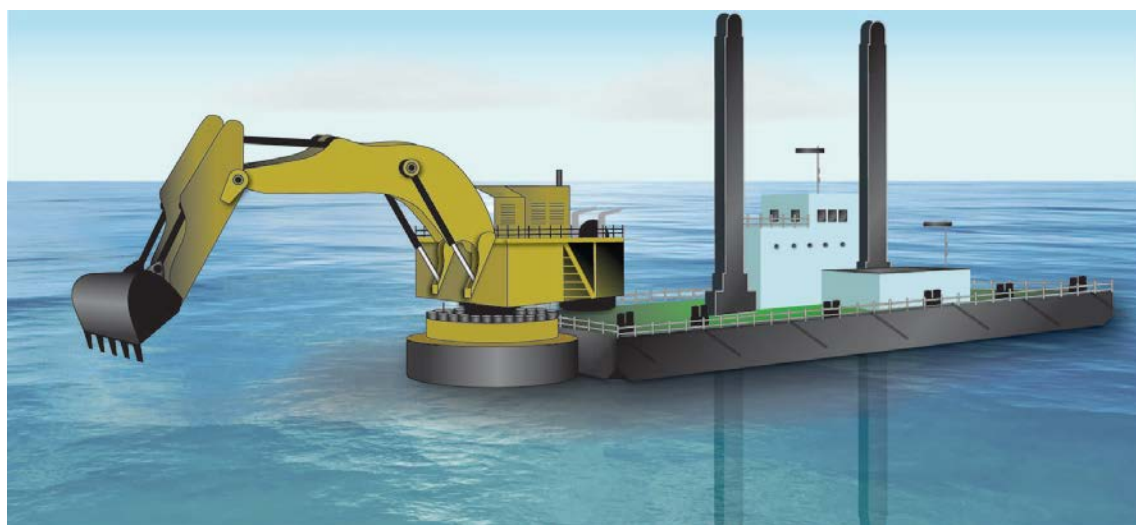
Figure 4.8: Schematic of Backhoe Dredger
