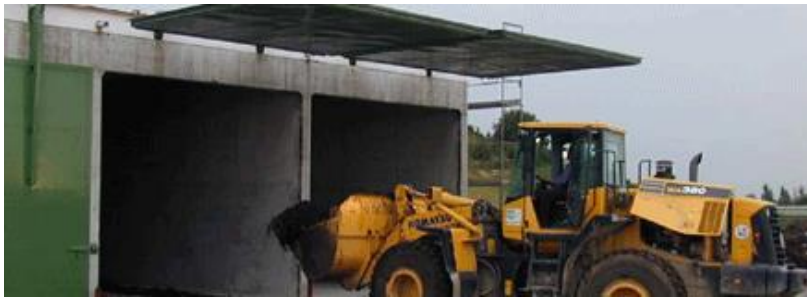
Figure 9: Ingestate loading systems: pipeline (top, source Veltrass) and wheel loader (down)
