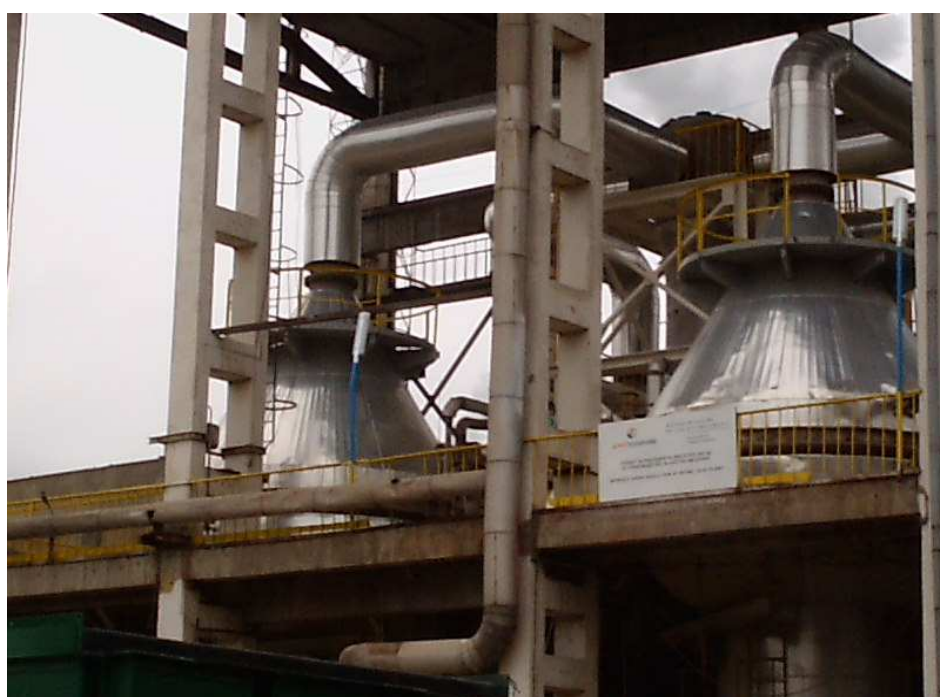
Figure 5 Two of the four reactors ( \text{NH}_3 burners)
