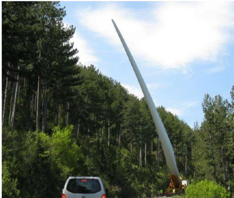
Figure 12: Transport of blades using a "bladelifter" vehicle
