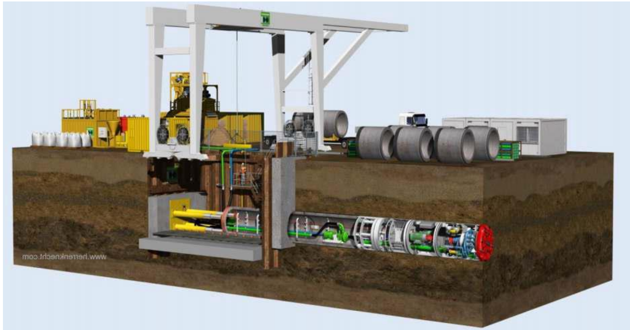
Figure 10.2 Presentation of the technological process of microtunnel execution
