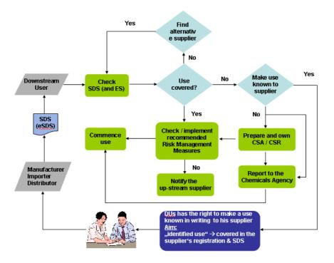
Figure 2 – Flowchart outlining Downstream User requirements
