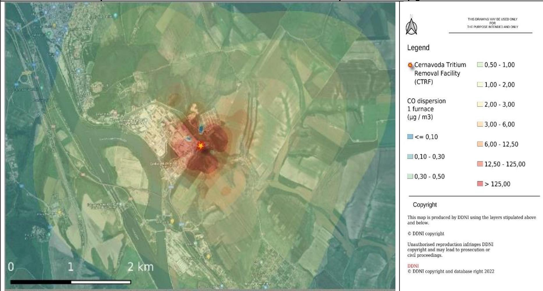
**Spatial distribution of CO concentrations under simultaneous operation of the 2 diesel units - back-up generator**
