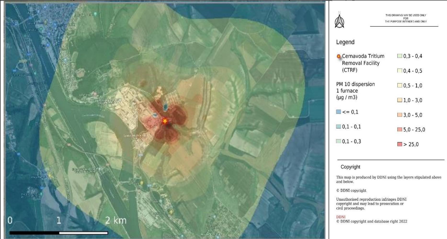
**Spatial distribution of PM<sub>10</sub> concentrations under simultaneous operation of the 2 diesel units - back-up generator**
