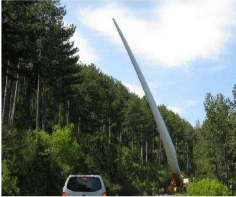
**Figure 2-12: Transporting blades using a bladelifter vehicle.**
