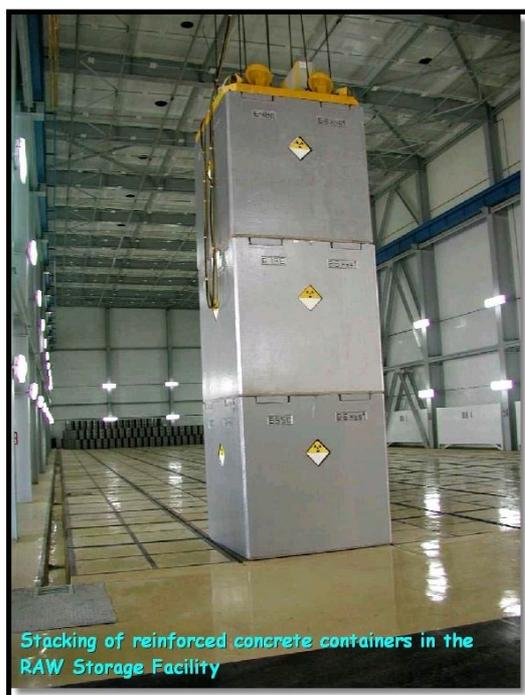
**FIGURE 2.2-4 REINFORCED CONCRETE CONTAINERS FOR DISPOSAL OF RAW IN NDF**
