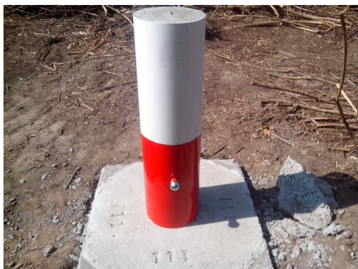
(a) an elevation benchmark bolt is installed on a survey marker
