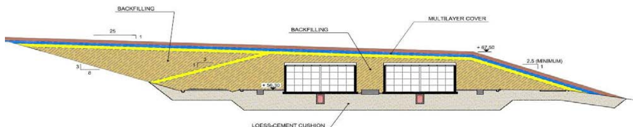
FIGURE 2.2-19 CROSS SECTION OF A CLOSED TRENCH-TYPE REPOSITORY
