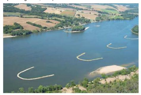
Figure II-13: Example of Chevrons (Source: US Army Corps of Engineers, 2008)
