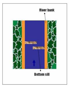
Figure 5.14: Two partial bottom sills (source: US Corps of Engineers, 2008)
