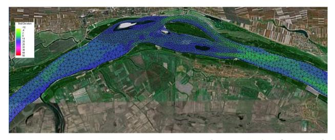
Figure III-10: Model grid and bathymetry at rkm630-620 (Aerial picture from Google.com).
