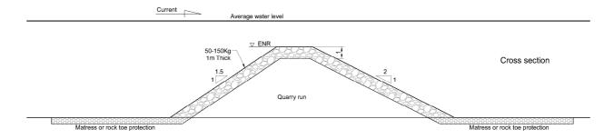
Figure II-14: Schematisation of a bottom sill (cross and longitudinal sections)
