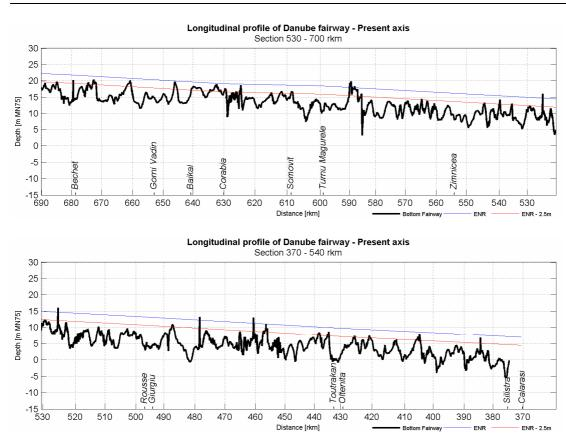
Figure III-1: Longitudinal profile along the current navigation channel rkm863-375
