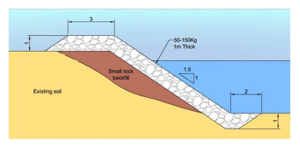
Figure III-11: Schematisation of a bank protection
