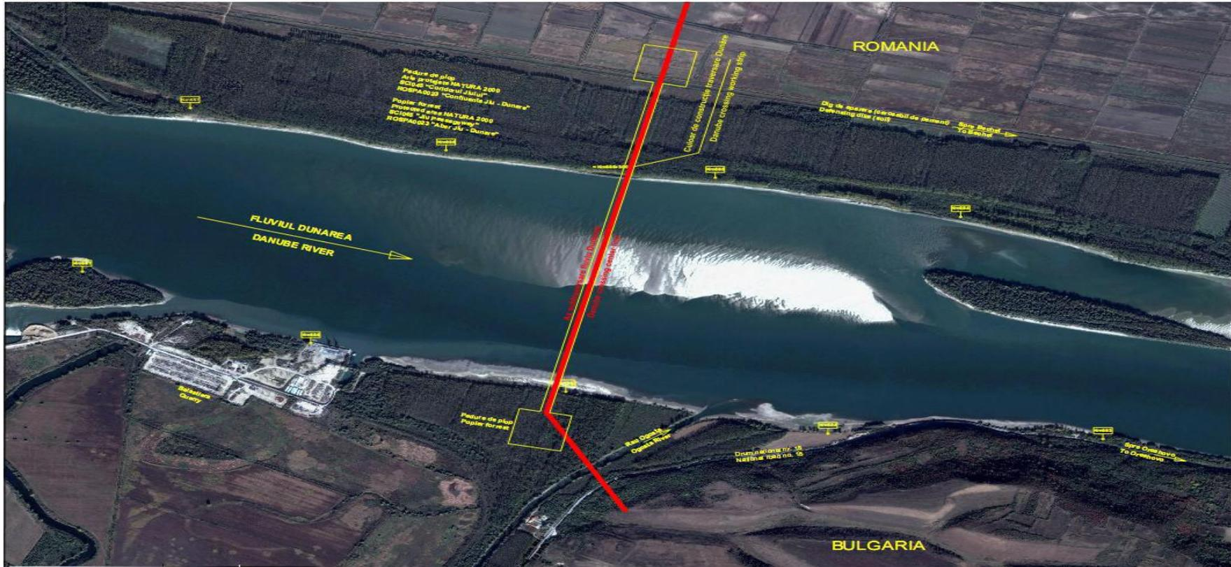
**Figure 2.9.:** Layout plan - the Danube crossing by trenchless method
