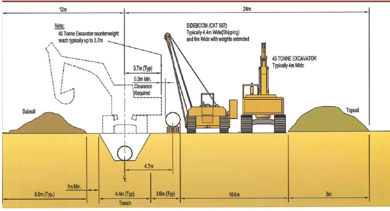
**Figure 2.10** : Typical drawings for execution of the trench.
