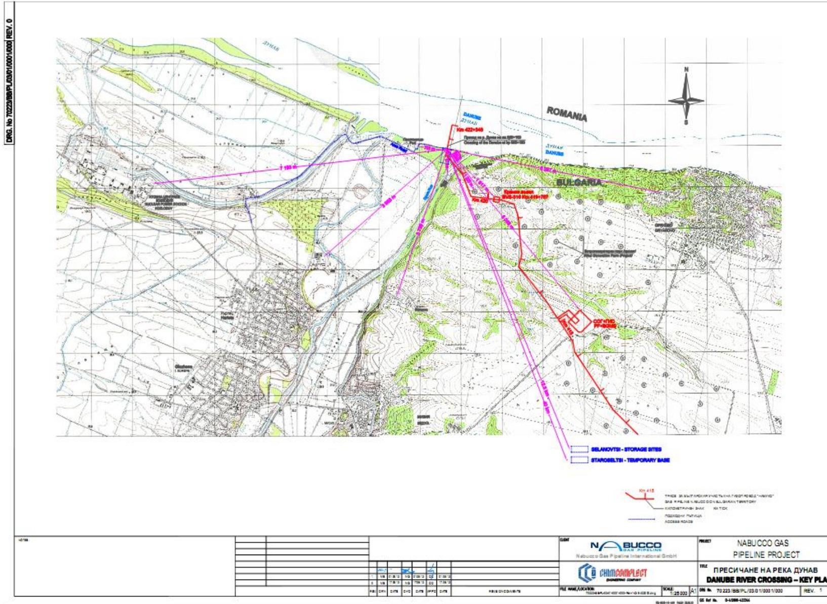
**Appendix 4 : Location of temporary construction camp and storage of excavated/dredged material/ drilling mud, depending on the Danube crossing method used**
