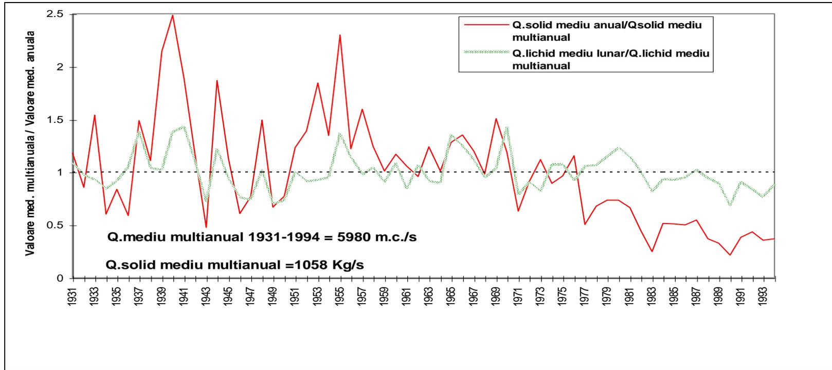
**Figure 5.2.5.** :Variation of medium annual liquid and solid flow during 1931-1994 at .Zimnicea H.S.
