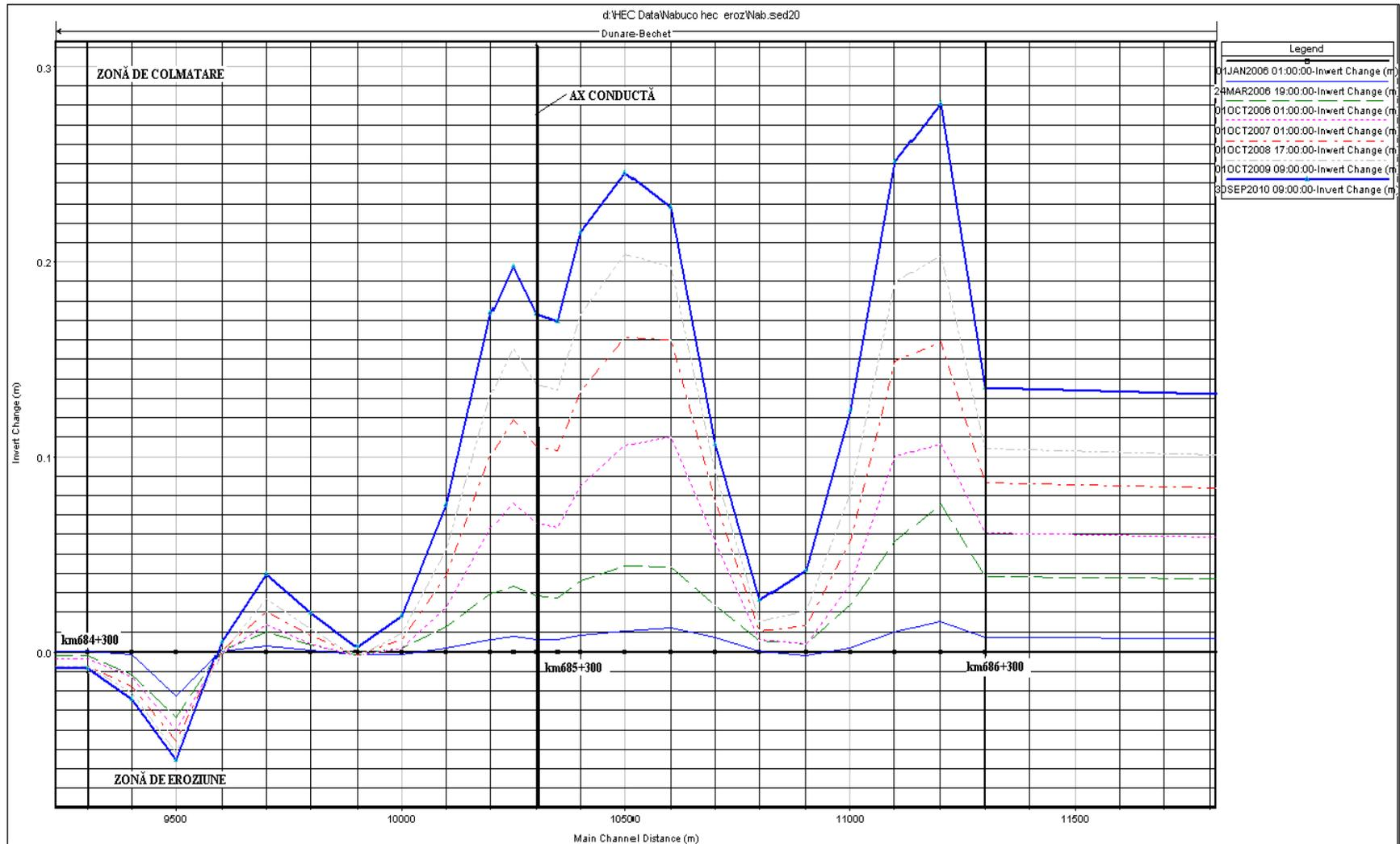
**Figure 5.2.10.:** Verification of the calculation model on the measured and calculated morphological evolution of the Danube riverbed, in the area of Bechet hydrometric station (km678+660) in 2005 and 2010.
