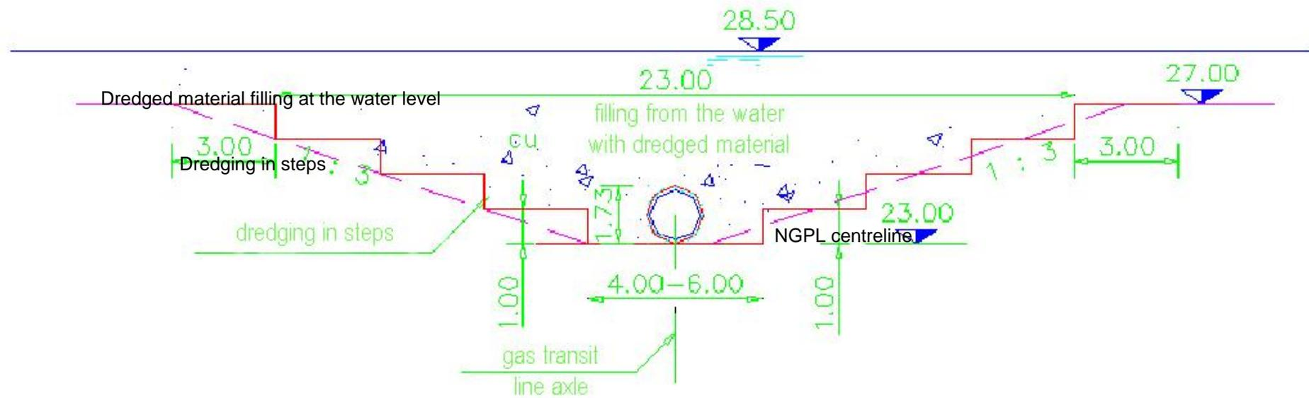
Figure A14.2...: Jiu river crossing. Current section in open cut option – red line: trench route
