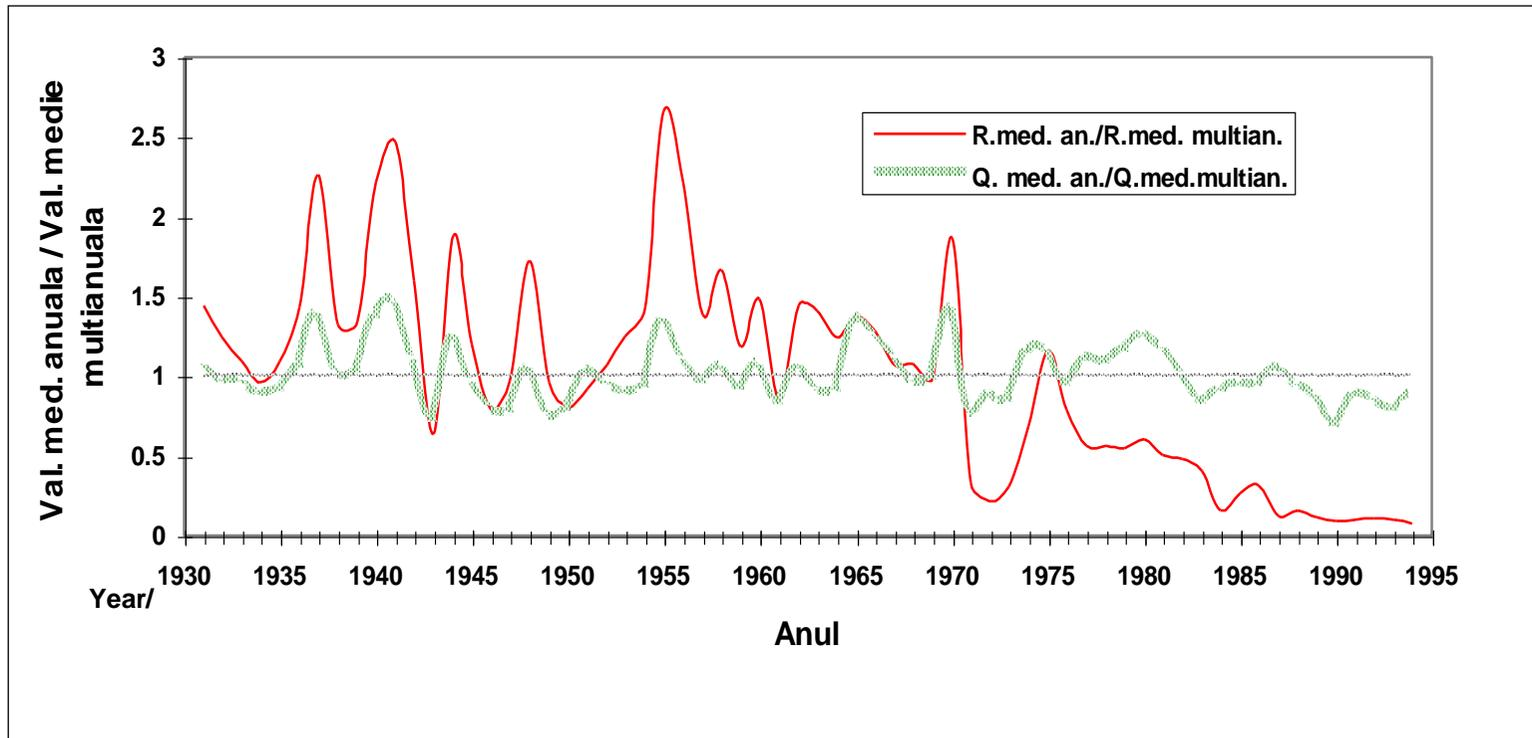
**Figure 5.2.4:** Variation of medium liquid and solid flow between 1931 – 1994 at H.S.Orsova
