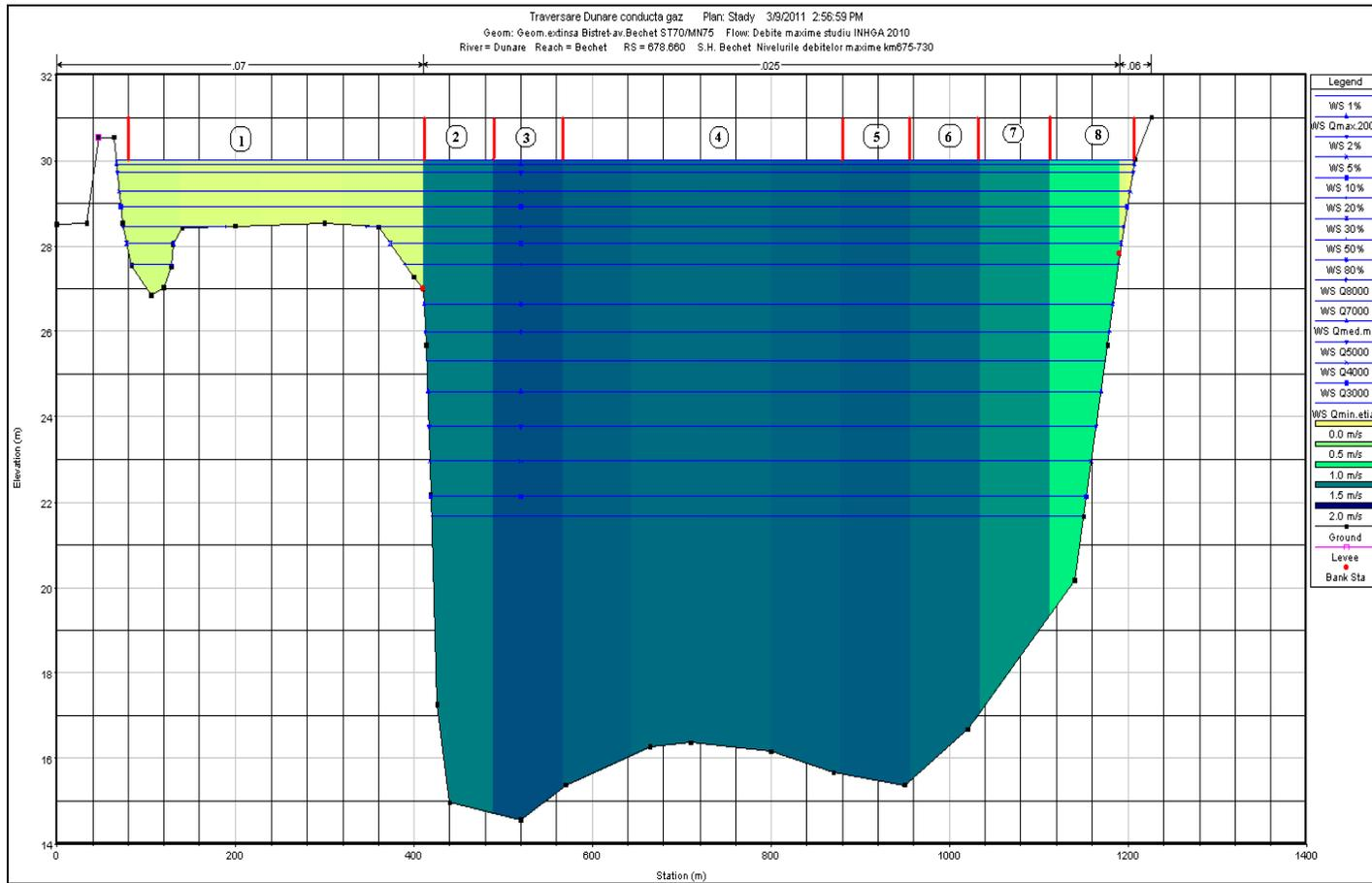
**Figure A12.3.:** Cross section of the Danube riverbed at Bechet H.S., km 678+660 and laying-out of specific data, rates of max. design flows, medium velocities on sectors
