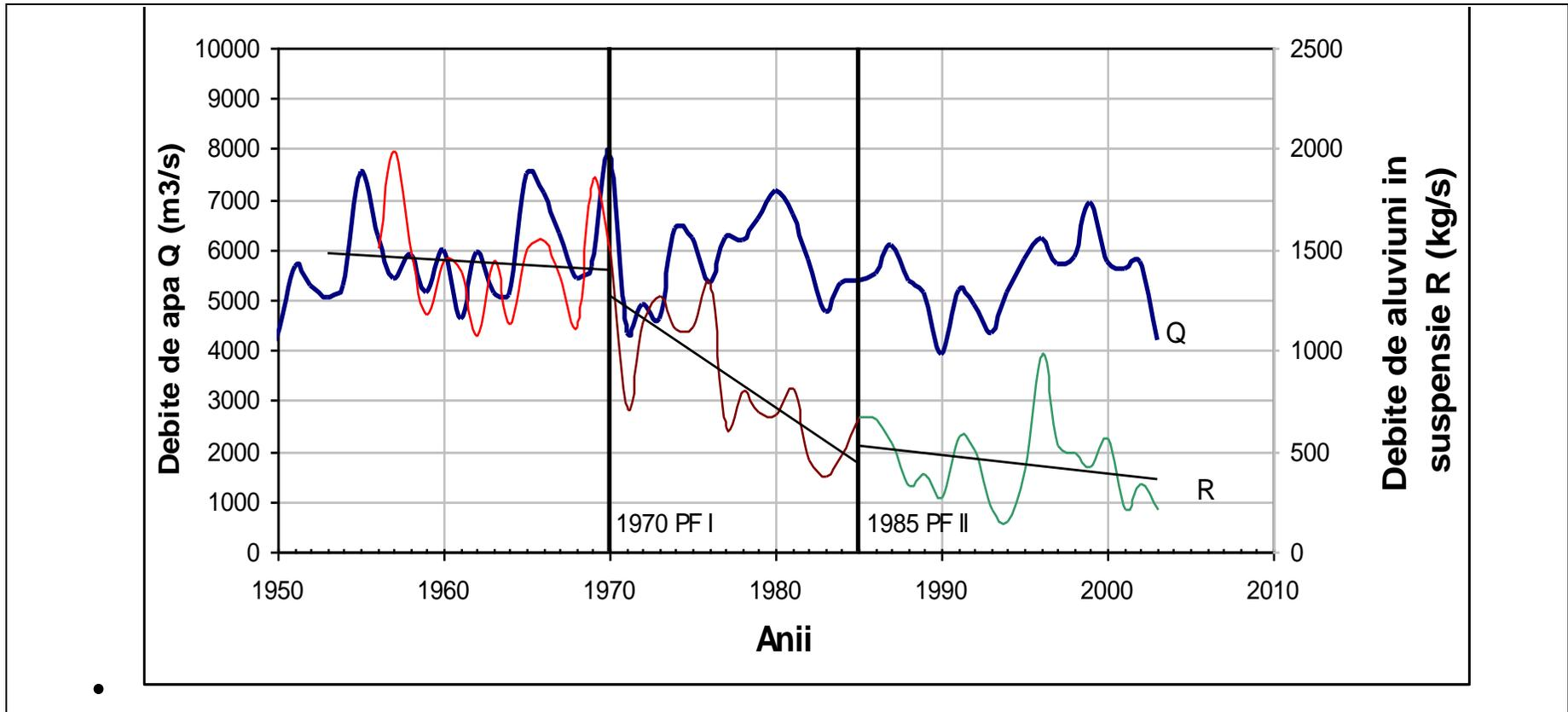
Figure 5.2.6.: Time variation of medium annual water and suspended sediment flows at Bechet H.S.
