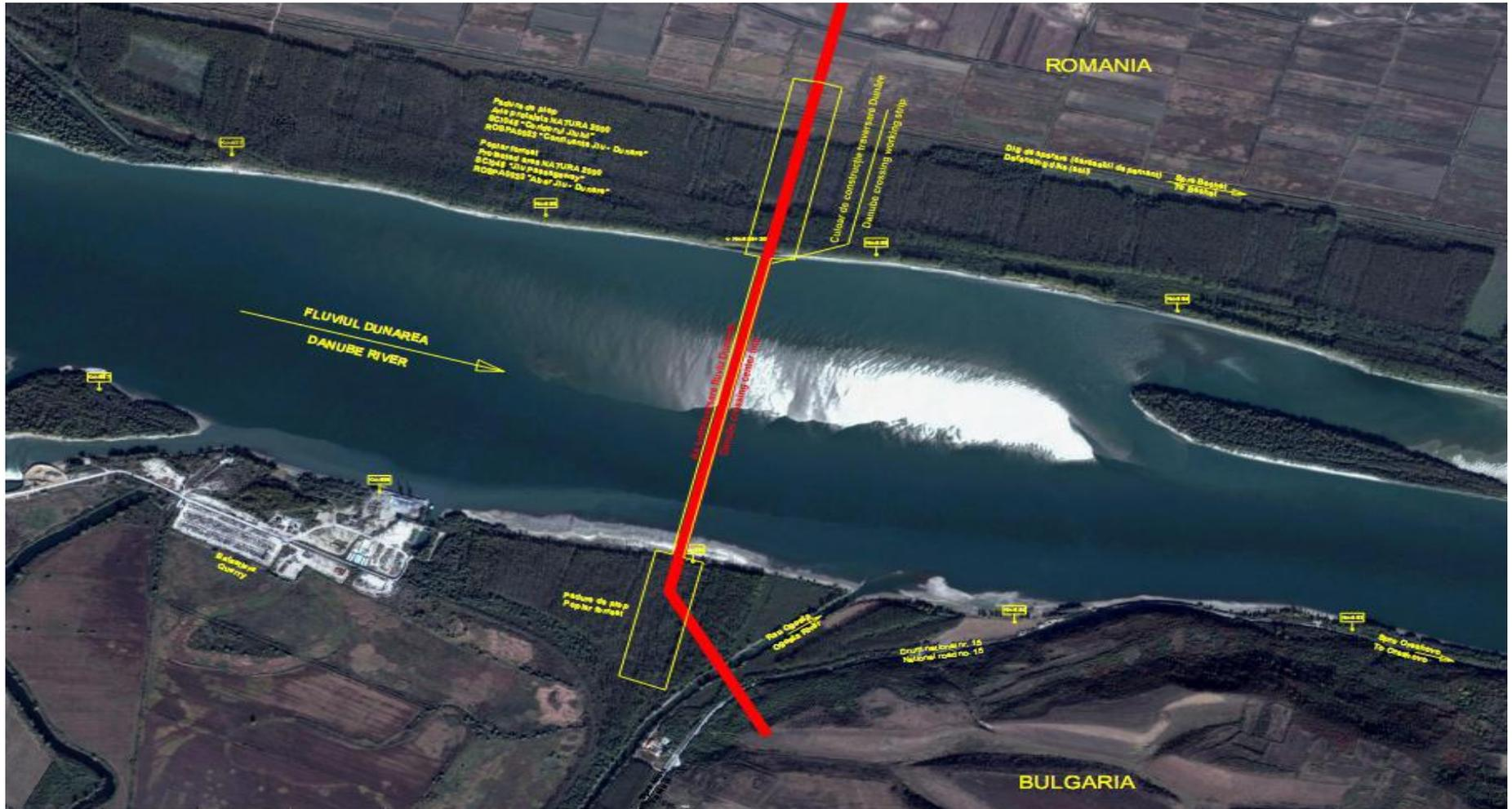
**Figure 2.8.:** Layout plan - the Danube undercrossing by open cut method
